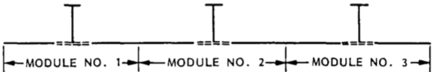
Fig. 1 Tee-stiffened panel with three modules. (From Computer Methods in Applied Mechanics and Engineering 103 (1993) 43-114)
