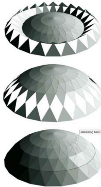
Figure 4 Schema of the of the pantadome erection
