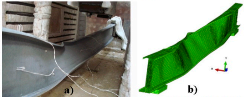
Figure 4.23 – Experimental (a) and numerical (b) configuration of the deformed lipped I beam with no restraints after fire test
