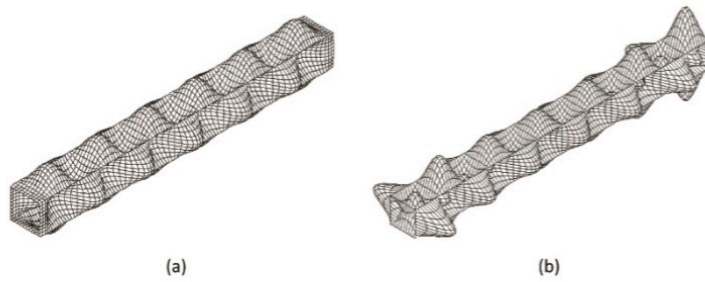
Fig. 8 Deformed shape of the empty tube under the pure compression after (a) collapse analysis (b) eigenvalue analysis
