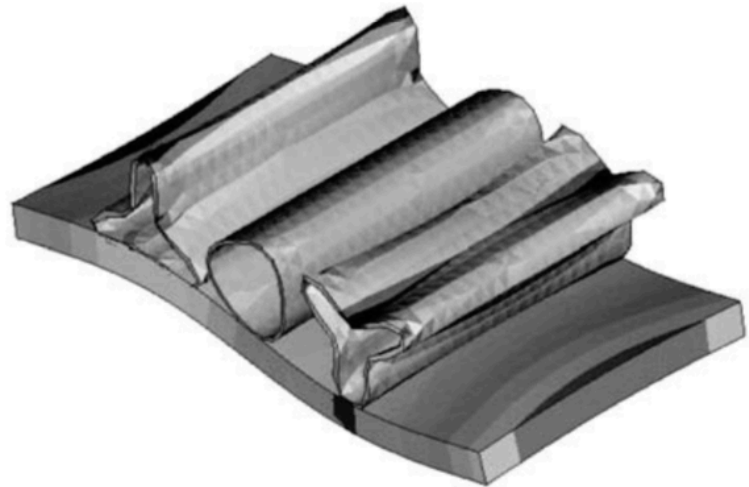
Fig. 3. Example of a high-frequency natural mode: vibrations of the substrate and nanotubes.
