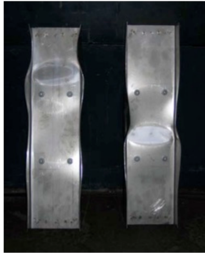
Figure 2.30. I304_500_1 and I304_500_2: Failed Shape
