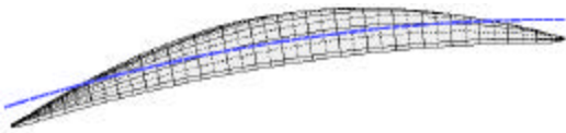
Fig. 16c First skin buckling mode in (a) viewed end on, demonstrating that the normal buckling modal displacement w is constant and non-zero along all four edges
