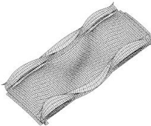
Fig. 16e Buckling in same STAGS model as (d) but with stiffener side-sway prevented at the edges
