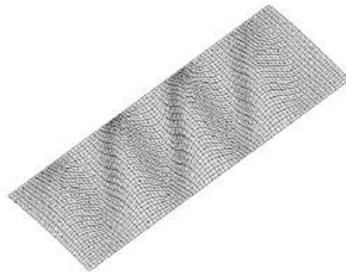
Fig. 16b Second skin buckling mode from the same STAGS model as in (a)
