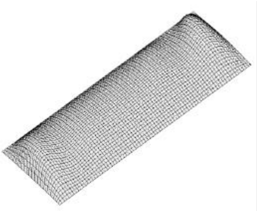
Fig. 16a First skin buckling mode from STAGS model type “1” with stringer model type “m” and ring model type “s” (Table 13)
