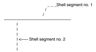
Segment 2 is joined to an internal point in Segment 1. You can always get the correct location of the connection of Shell segment no. 2 to Shell segment no. 1 if, instead of using two shell segments, you divide the same geometry into three shell segments, as in the sketch below:
