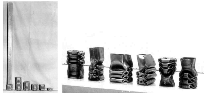
Fig. 6. Progressive folding of properly triggered prismatic members subject to the predominantly axial crash loading.
