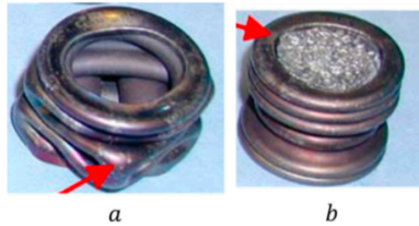
Fig. 6 Diamond and concertina deformation modes of (a) empty- (b) foam-filled long tubes. Reproduced from Asakavithchai, S., Slater, D., Kennedy, A.R., 2004. Effect of tube length on the buckling mode and energy absorption of Al foam-filled tubes. J. Mater. Sci. 39 (24), 7395-7396.
