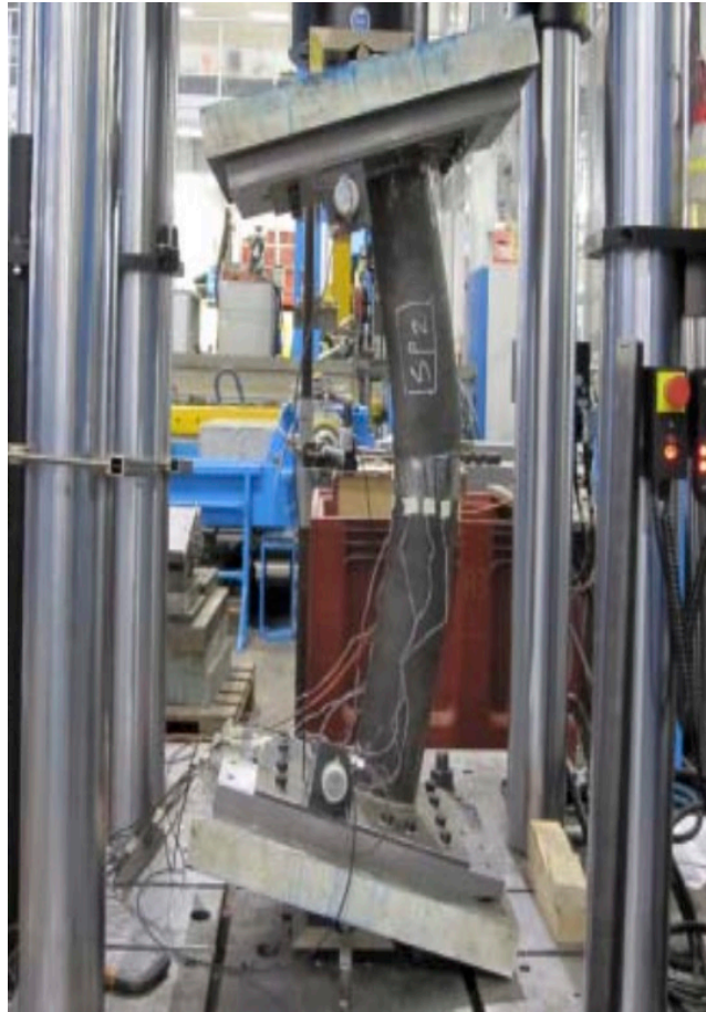
Structural lab testing facility for column buckling
