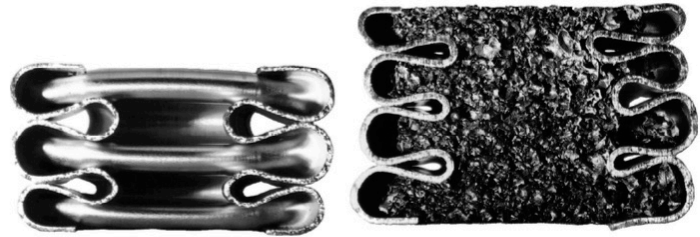
Figure 6 Axial crushing of non-filled and foam-filled circular and square extrusions, quasi-static loading
