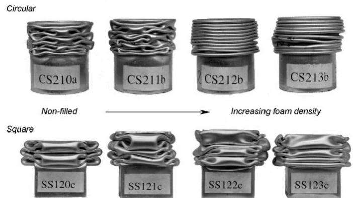
Figure 6 Axial crushing of non-filled and foam-filled circular and square extrusions, quasi-static loading
