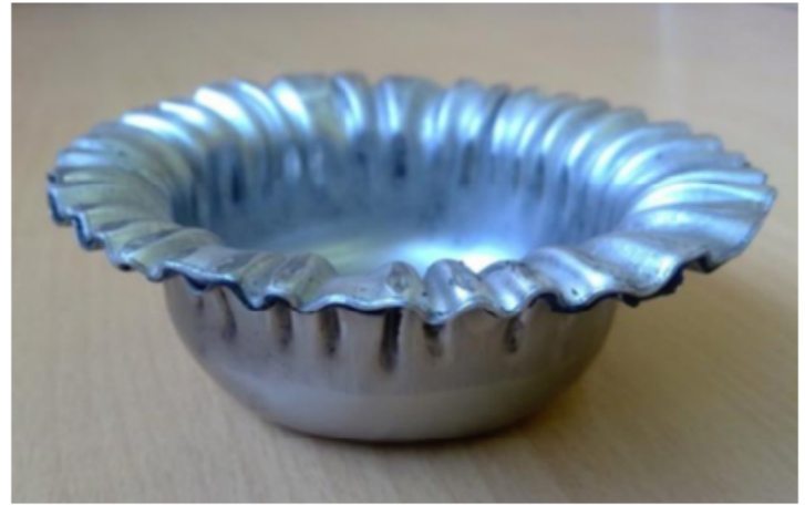
Figure 3. Sample of laminated sheet after forming.
