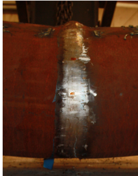
[Buckling of thin-walled concrete-filled tube]
