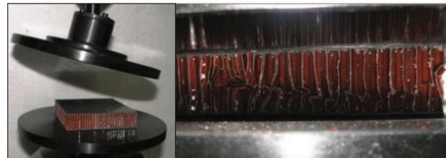
Fig. 4. Compression test set-up and compressed specimen.
