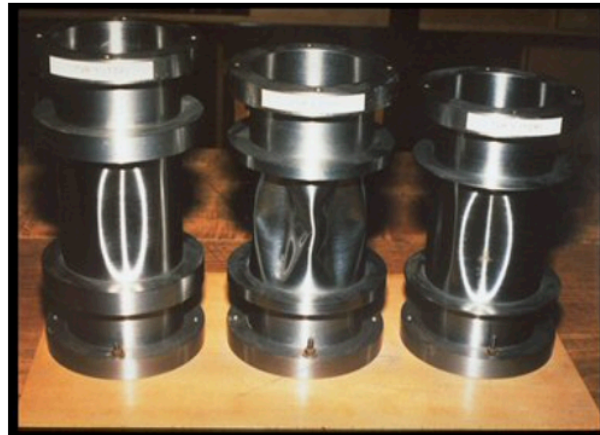
Figure 1, Shell instability of a circular cylinder
