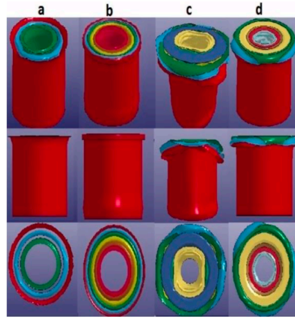
Fig. 4. Isometric, front and top view of all samples after deformation processes a) n=1 , b) n=2 , c) n=3 and d) n=4
