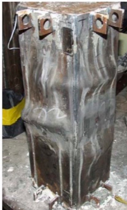
Fig. 12 Typical short column failure from test series
