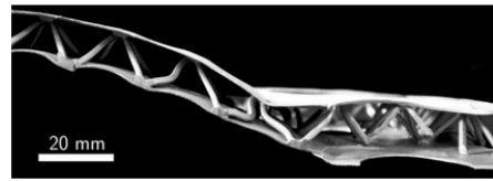
(b) detail of buckled truss members
