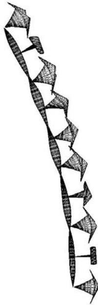
End view of STAGS model with rings removed so that skin-stringer buckling shows
