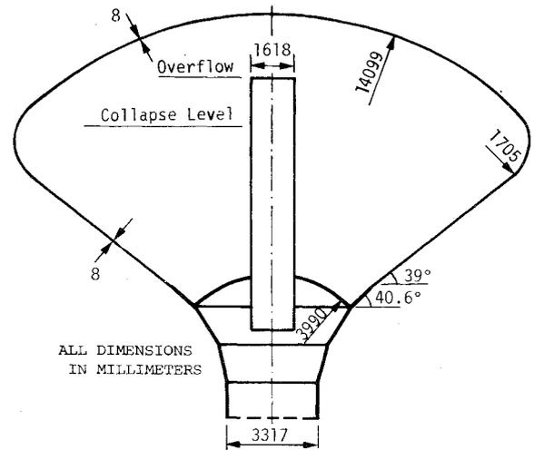
Fig. 1.4 Geometry of large steel water tank that failed in Belgium in 1972 (from Vandepitte<sup>3</sup>).
