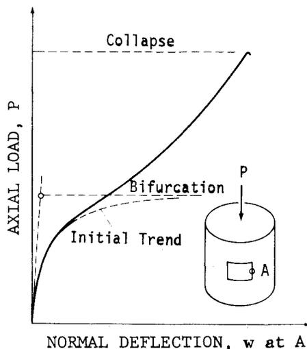
Fig. 4.3 Equilibrium paths for axially compressed cylindrical shell with two diametrically opposed cutouts. (From *Buckling of Bars, Plates, and Shells* by D. O. Brush and B. O. Almroth.<sup>11</sup> Copyright © 1975 by McGraw-Hill, Inc. Used with permission of McGraw-Hill Book Co.)
