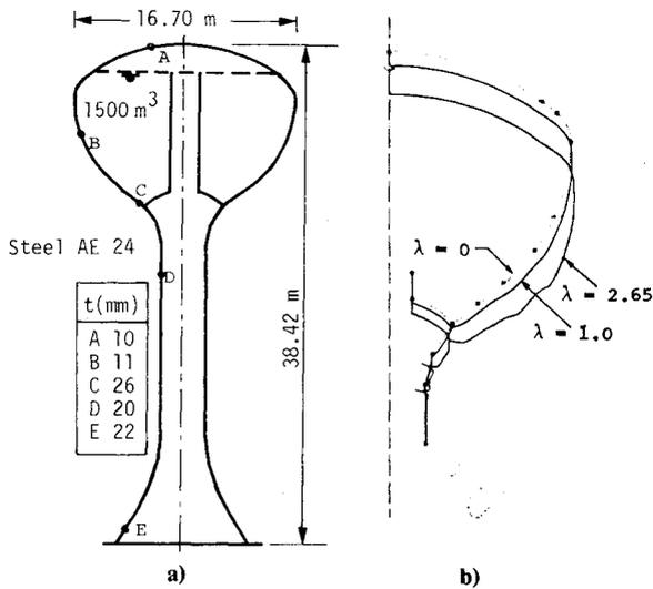
Fig. 9.3 New design of the water tank and axisymmetric deformation at load factor,  $\lambda=2.65$ , which corresponds to predicted collapse (from Baltus and Massonnet<sup>2</sup>). a) New design; b) predicted deformation of new design at collapse.
