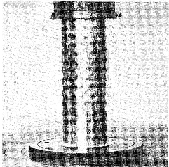
Fig. 3.1 Cylinder with completely developed elastic buckle pattern (from Horton et al.<sup>44</sup>).
