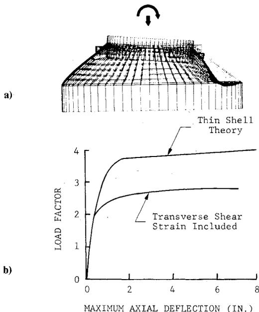
**Fig. 6.6 Collapse of stiffened conical shell with sandwich wall construction (from Sharifi<sup>48</sup>). a) Deformation at collapse. b) Collapse load factors with and without transverse shear deformation effects.**
