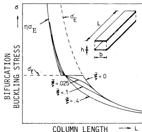
Fig. 7.7 Column buckling load for two-flange model of given cross section as function of column length and flange imperfection amplitude. This configuration was studied by van der Neut<sup>171</sup> and Thompson and Lewis<sup>172</sup> (from Tvergaard<sup>168</sup>).
