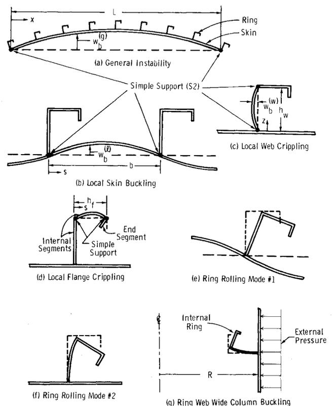
**Fig. 7.1 General and local bifurcation buckling modes for a stiffened panel.**
