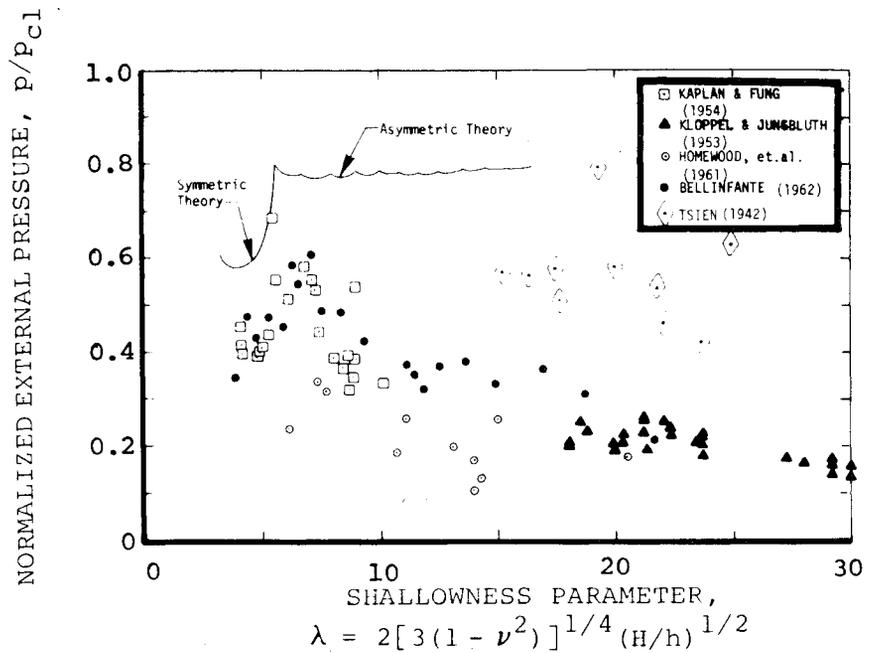
Fig. 3.11 Early experimental results for clamped spherical caps under external pressure ( $H$  is the rise of the apex of the cap above its base plane). [From Fung and Sechler, *Thin Shell Structures: Theory, Experiment and Design*, © 1974, p. 253. Reprinted by permission of Prentice-Hall, Inc., Englewood Cliffs, N.J. (Kaplan<sup>43</sup>).]
