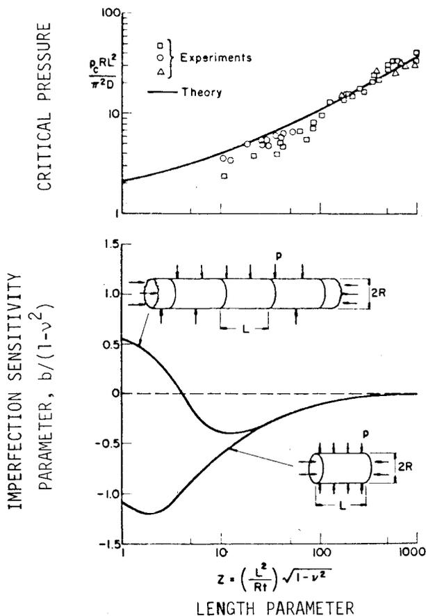
Fig. 3.13 Comparison between test and classical theory and initial postbuckling predictions for externally pressurized cylinders (from Hutchinson and Koiter<sup>16</sup>).
