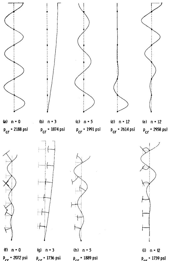
**Fig. 7.5** Predicted buckling pressures and modes of internally ring-stiffened cylindrical shell. (a-e) T-shaped rings treated as discrete (cross sections cannot deform). (f-i) T-shaped rings treated as flexible shell segments (cross sections deformable).
