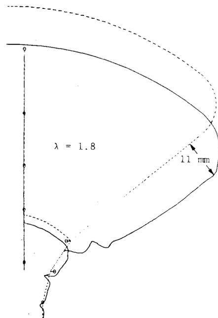
**Fig. 9.2 Axisymmetric deformation of steel water tank at load factor corresponding to predicted collapse ( $\lambda = 1.0$  corresponds to actual collapse conditions existing in 1972 at the time of the disaster).**
