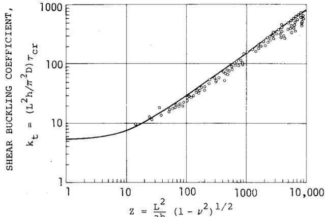
Fig. 3.8 Comparison of theoretical and experimental buckling loads for cylinders subjected to torsion. (From *Buckling of Bars, Plates, and Shells* by D. O. Brush and B. O. Almroth.<sup>11</sup> Copyright © 1975 by McGraw-Hill, Inc. Used with permission of McGraw-Hill Book Co.)
