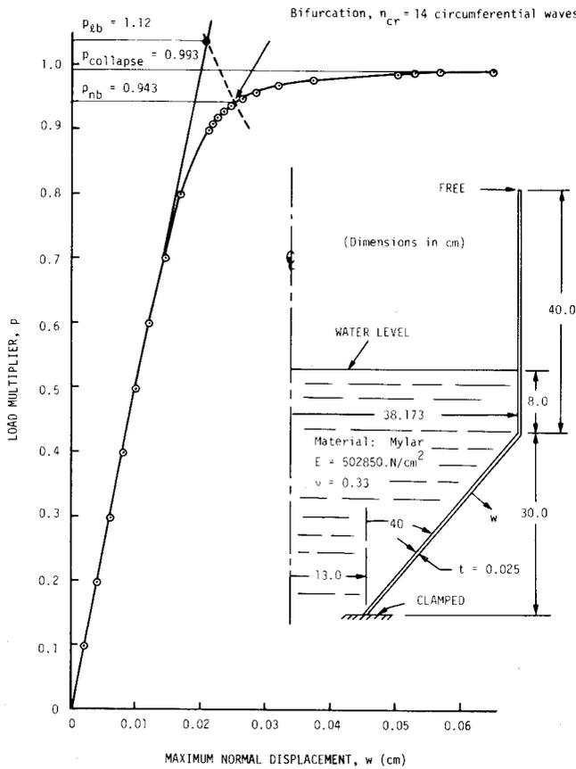
**Fig. 1.6** Load-maximum-normal-deflection curve for conical water tank, with bifurcation points  $P_{bb}$  from linear and  $P_{nb}$  from nonlinear prebuckling theory and axisymmetric collapse load factor,  $P_{collapse}$ .
