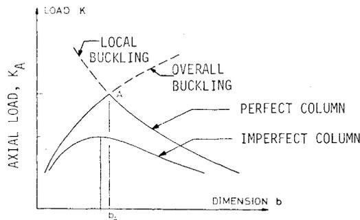
Fig. 7.8 Degeneration of an optimum design because of imperfections (from Thompson and Lewis<sup>172</sup>).
