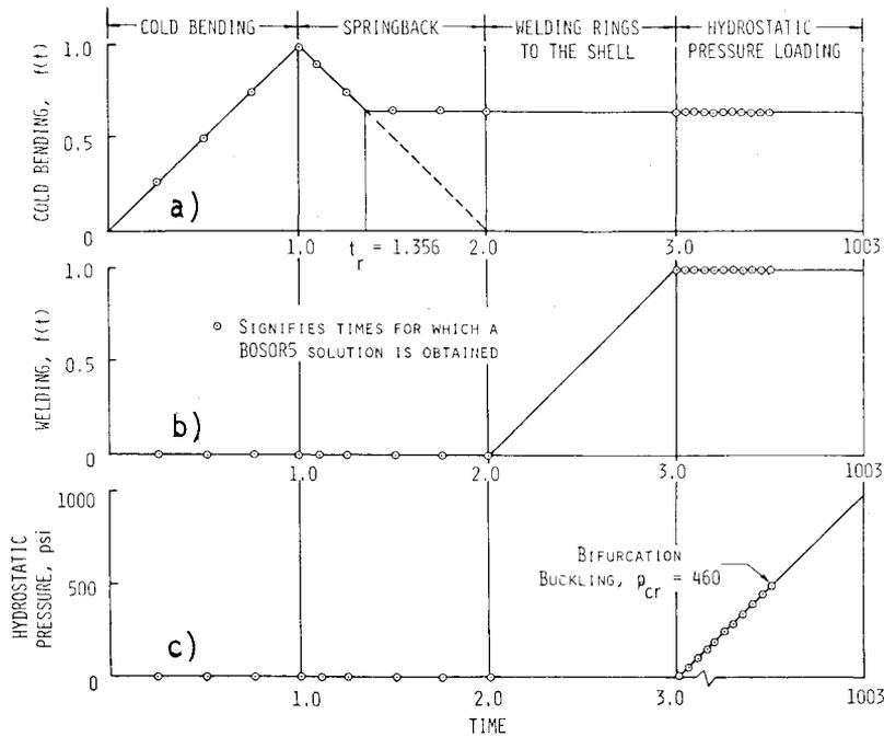
Fig. 5.11 Loading functions of "time" for BOSOR5 analysis of the fabricated ring-stiffened cylinder BR-4: a) cold-bending process; b) welding the rings to the cylinder; c) application of the external hydrostatic pressure.
