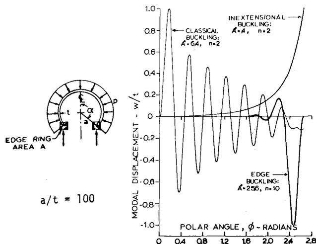
Fig. 6.1 Buckling modes for an externally pressurized spherical shell with an edge ring of dimensionless area  $A^* = (A/at)(a/t)^{1/2} = 0.4, 6.4,$  and  $25.6$  (from Bushnell, *AIAA Journal*, Vol. 5, 1967, p. 2046).
