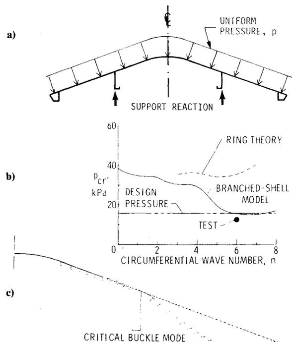
Fig. 7.3 Buckling of lightweight ring-stiffened shallow conical shell designed by NASA for decelerating a payload entering the Martian atmosphere (from Leonard et al.<sup>137</sup>). a) Loading; b) comparison of buckling test and predictions from two analytical models; c) critical buckling mode, showing interaction of general buckling and local deformation of rings.
