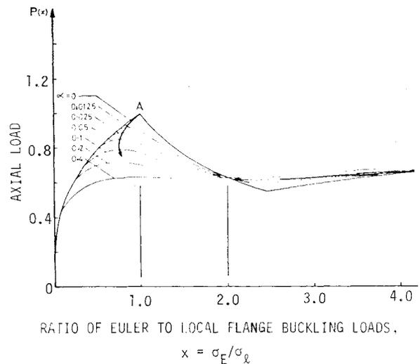
Fig. 7.9 Erosion of the optimum load of the two-flange column shown in Fig. 7.7 by initial flange imperfections  $\alpha$  (from Thompson and Lewis<sup>172</sup>).
