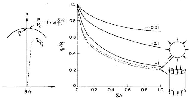
Fig. 3.3 Imperfection sensitivity as a function of parameter  $b$  for unique buckling mode and comparison with imperfection sensitivity of spherical shell under external pressure and cylindrical shell under axial compression;  $\delta$  is the amplitude of the buckling mode and  $\bar{\delta}$  is the amplitude of the imperfection (from Budiansky and Hutchinson<sup>53</sup>).
