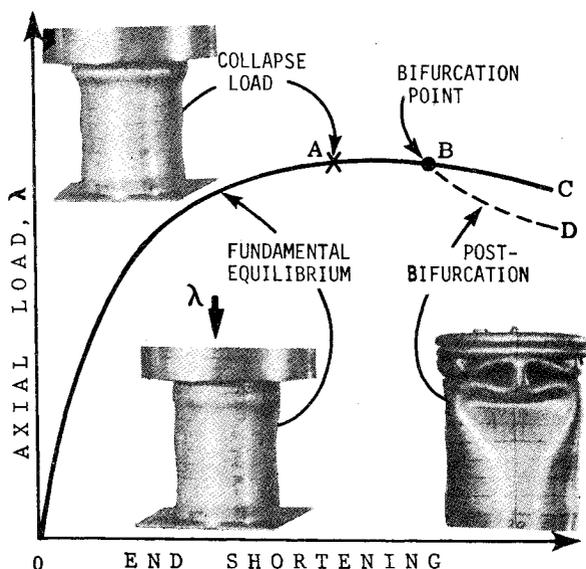
Fig. 2.1 Load/end-shortening curve with collapse load A, bifurcation point B, and postbifurcation equilibrium path BD (photographs courtesy of Sobel and Newman<sup>87</sup>).
