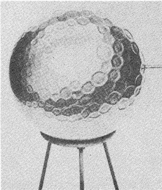
Fig. 3.9 Postbuckled state of a thin-walled spherical shell under uniform external pressure; buckling motion is restrained by an interior mandrel (from Carlson et al.<sup>45</sup>).
