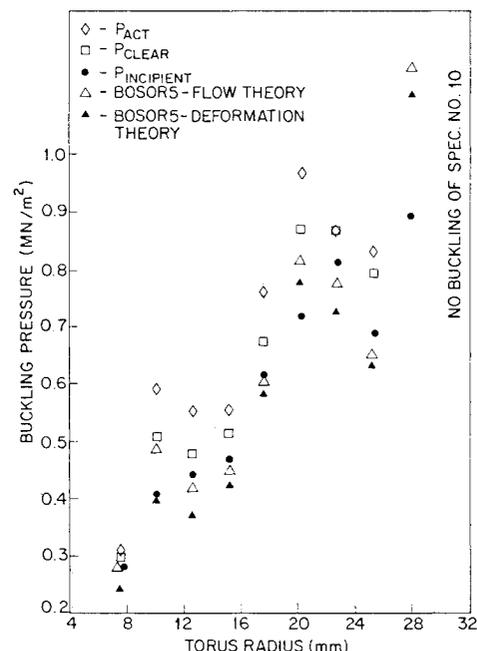
Fig. 5.8 Variation in buckling pressure with radius of toroidal knuckle: comparisons of test results of Ref. 108 with BOSORS predictions for incipient buckling (from Lagae and Bushnell<sup>104</sup>).
