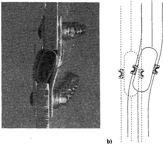
Fig. 9.4 Failure of axially compressed frangible joint typical of those used in rockets for the separation of booster stages (from Bushnell<sup>186</sup>). a) Test specimen, b) BOSOR6 hybrid model.
