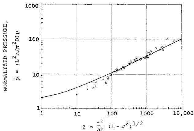
Fig. 3.6 Comparison of theoretical and experimental buckling pressures for cylinders subjected to external hydrostatic pressure ( $D$  = flexural rigidity). (From *Buckling of Bars, Plates, and Shells* by D. O. Brush and D. O. Almroth.<sup>11</sup> Copyright © 1975 by McGraw-Hill, Inc. Used with permission of McGraw-Hill Book Co.)
