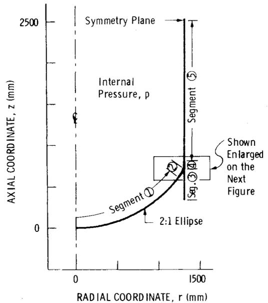
**Fig. 5.1 Bottom part of rocket fuel tank as modeled for input to the BOSOR4 computer program.**
