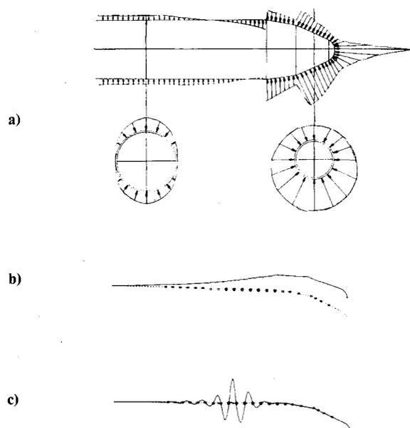
Fig. 6.2 Nonsymmetric pressure loading on the payload shroud shown in Figs. 1.9a and 1.9b (from Bushnell<sup>9</sup>). a) Pressure distribution. b) Prebuckling beam-type deflection. c) Nonsymmetric buckling mode.  $n_{cr} = 13$  circumferential waves.
