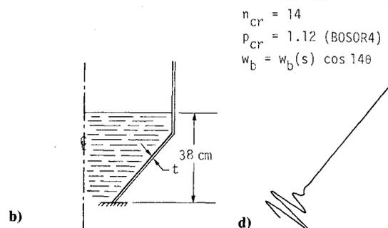
Fig. 1.5 Elastic buckling of conical water tank: a) specimen before buckling; b) tank geometry and water level; c) postbuckled specimen; and d) predicted bifurcation buckling load factor and mode from linear theory (photographs courtesy of Dr. G. Lagae, University of Ghent, Belgium).
