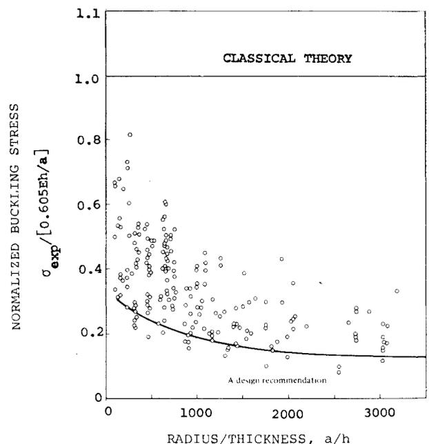
Fig. 3.2 Distribution of test data for cylinders subjected to axial compression. (From *Buckling of Bars, Plates and Shells* by D. O. Brush and B. O. Almroth.<sup>11</sup> Copyright © 1975 by McGraw-Hill, Inc. Used with permission of McGraw-Hill Book Co.)
