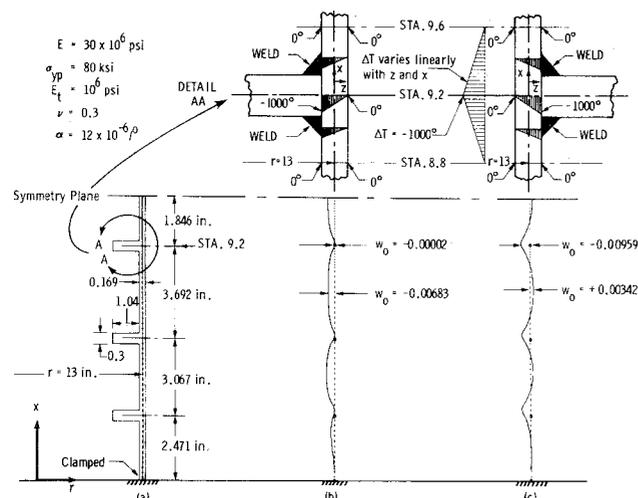
**Fig. 5.9** Cylinder with welded internal and external rings: a) dimensions and BOSOR5 discretized reference surface; b) predicted residual deformations after welding and before loading of specimen with internal rings; c) predicted residual deformations after welding and before loading of specimen with external rings.
