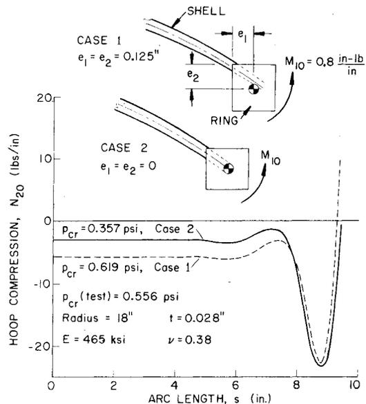
Fig. 6.5 Effect of edge ring eccentricity on predicted buckling pressures of shallow spherical cap (from Bushnell<sup>143</sup>).
