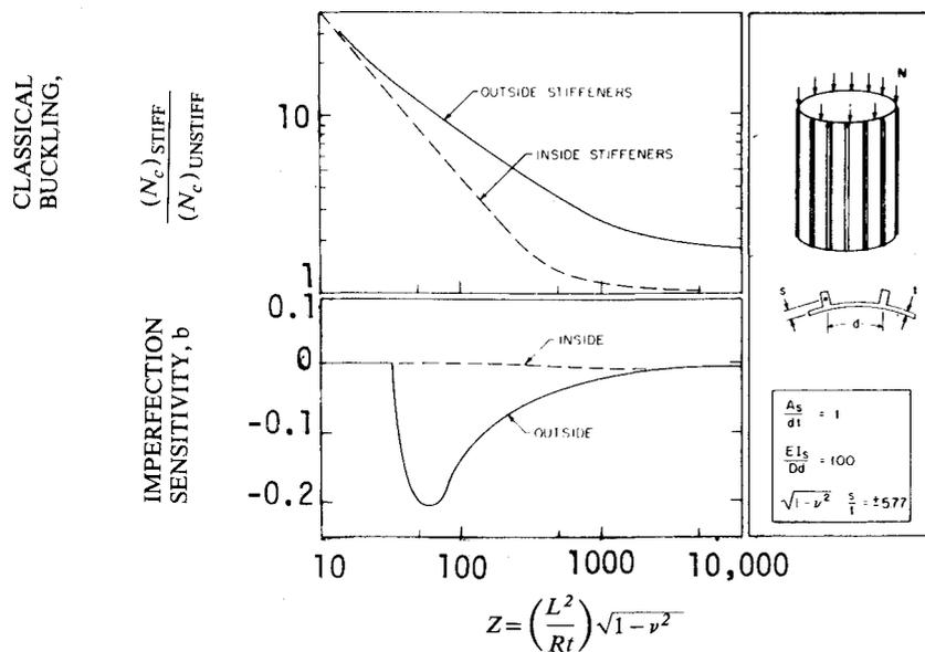
Fig. 3.12 Classical buckling and imperfection sensitivity of simply supported stiffened cylinders under axial compression (from Budiansky and Hutchinson<sup>53</sup>).
