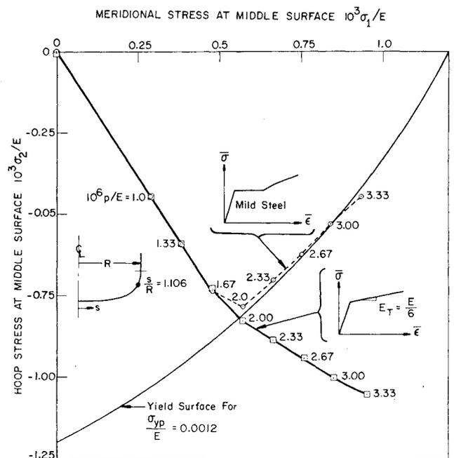
Fig. 5.6 Comparison of paths in stress space at station  $s/R = 1.106$  with increasing internal pressure in ellipsoidal heads with two different hardening moduli (from Bushnell, *Transactions of ASME, Journal of Pressure Vessel Technology*, Vol. 99, Feb. 1977, p. 63).
