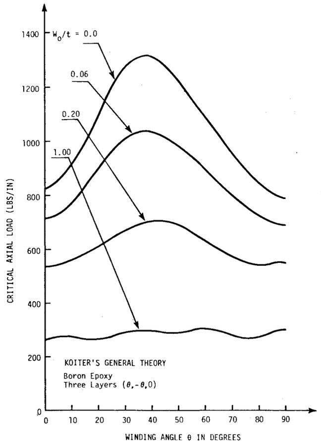
Fig. 3.14 Effect of initial imperfection amplitude  $w_0$  on the buckling load of a composite cylinder; predictions are from Koiter's general theory, obtained by Khot and Venkayya.<sup>67</sup> (From Almroth<sup>70</sup>.)
