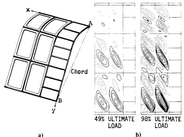
**Fig. 6.7 Computer analysis of shear panel (from Skogh and Stern<sup>151</sup>). a) Complex stiffened shear panel. b) Postbuckling behavior predicted with the STAGS computer program.**
