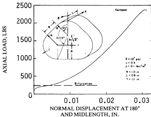
Fig. 4.5 Noncircular cylinder subjected to uniform end shortening (from Almroth and Brogan<sup>97</sup>).
