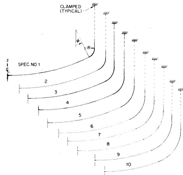
Fig. 5.7 Discretized models of torispherical heads under internal pressure tested by Patel and Gill<sup>108</sup> (from Lagae and Bushnell<sup>104</sup>).
