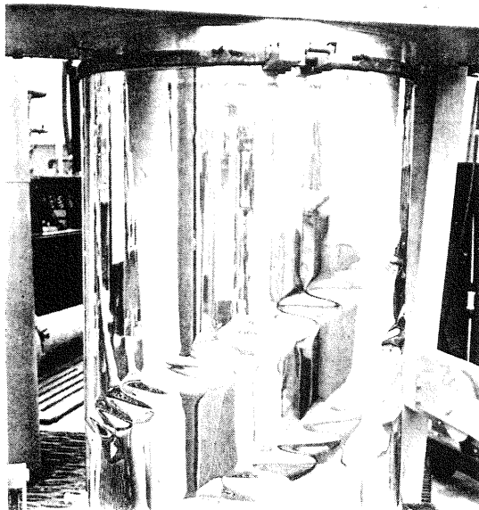
Fig. 5—Typical buckle pattern for pressurized cylinder in compression
