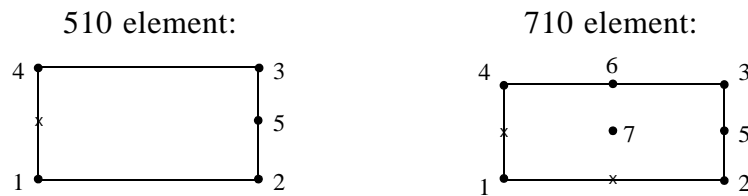
Figure 14.13 Node numbering for mesh-transition elements
